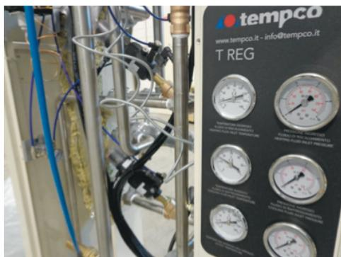
*The recirculation circuit is usually constructed in pressurised version. The atmospheric version is also available, where the upper temperature limit cannot exceed 95°C. On request, the units can be constructed in explosion-proof ATEX version for explosive environments.*
