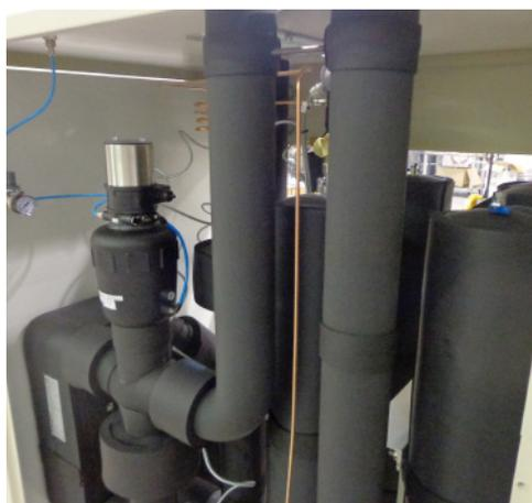
*On the outside are shut-off valves on the service fluids as well as on the fixture. The front instrument panel assures total control over the unit, and the REM option makes it possible to monitor and control all unit functions from a remote station. The type of reporting and communication protocol may be optionally defined. All internal pipes are in AISI 304 stainless steel. Insulation may be provided on request.*
